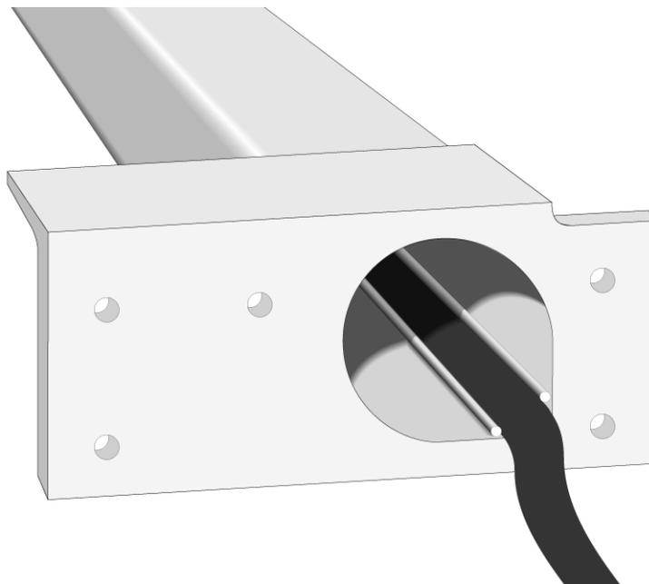
18. Using a broom handle or other long, narrow object, press the ribbon cable into the cable channel that runs the length of the lift column.
