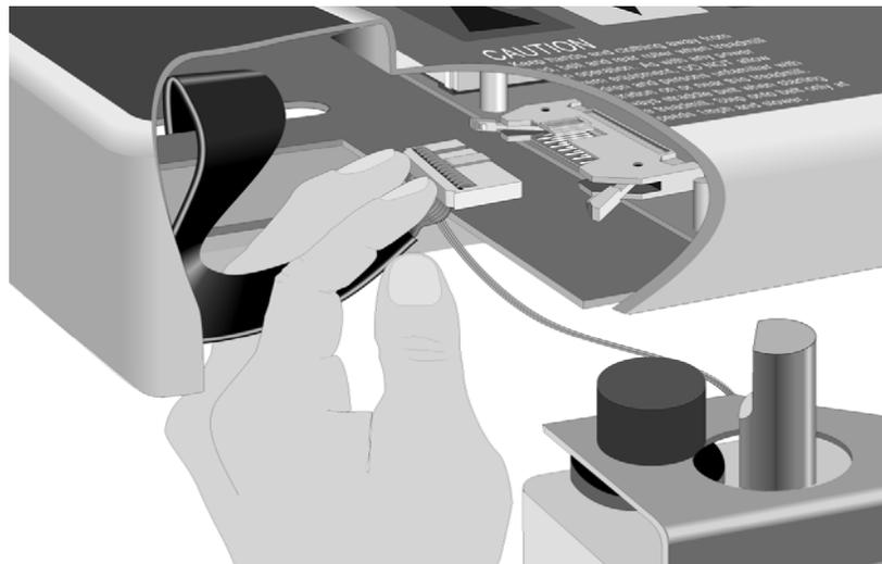
8. Attach the wrist strap to your arm, then connect the ground lead of the wrist strap to the treadmill frame.
