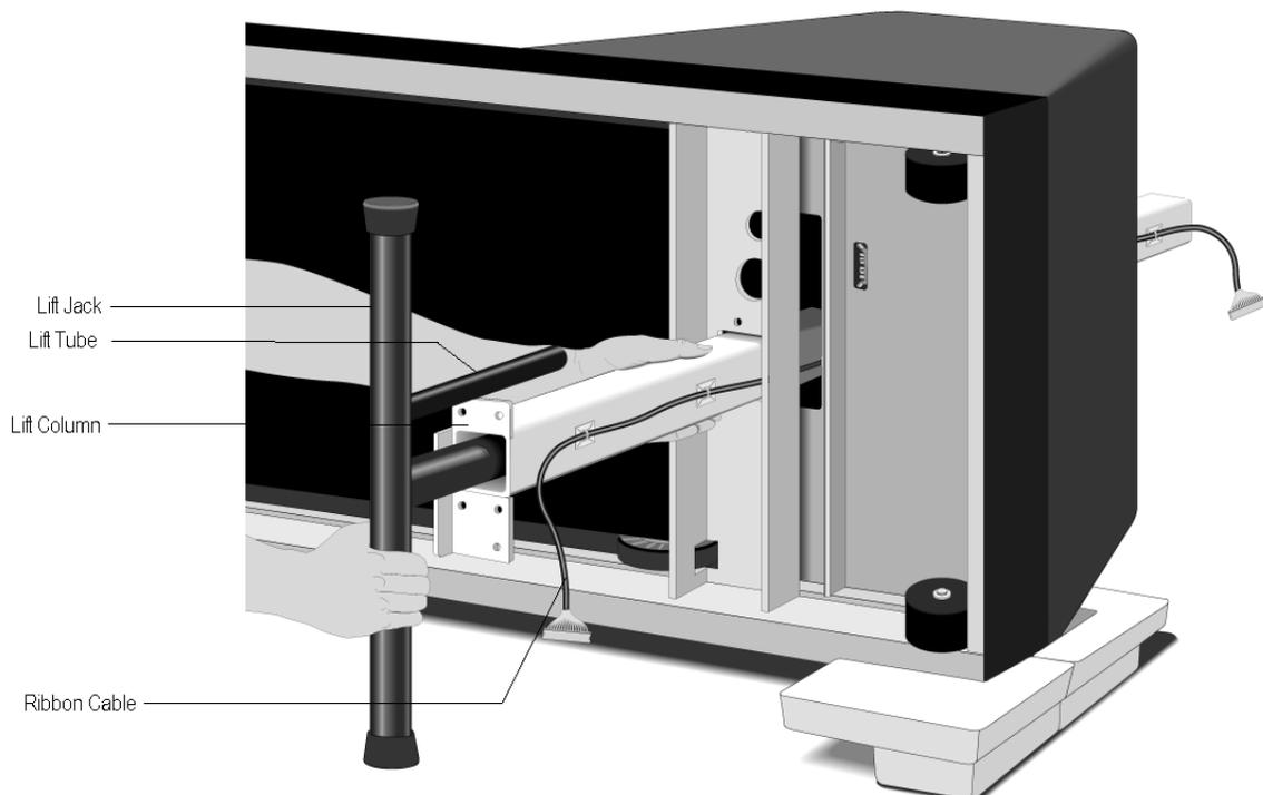
17. Slide the lift column through the base of the treadmill frame.
