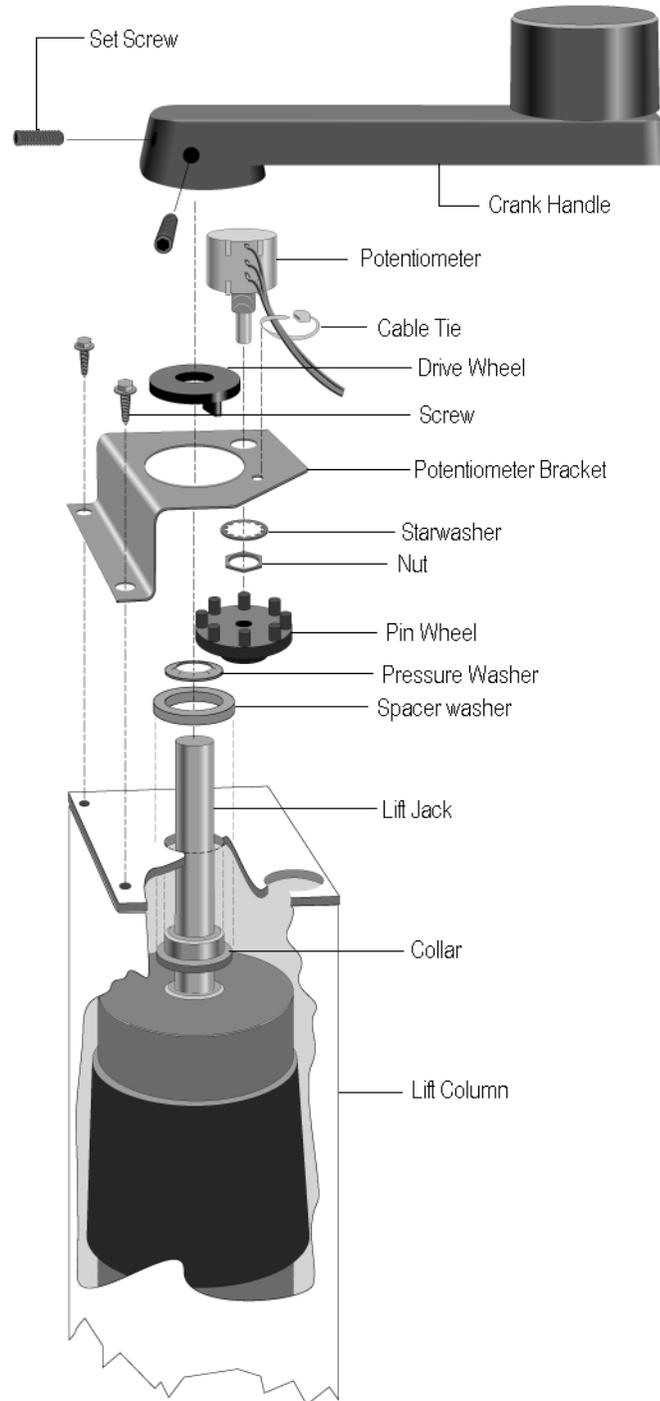
12. Pull the lift jack from the lift column and set it aside (see Diagram 6.9).
