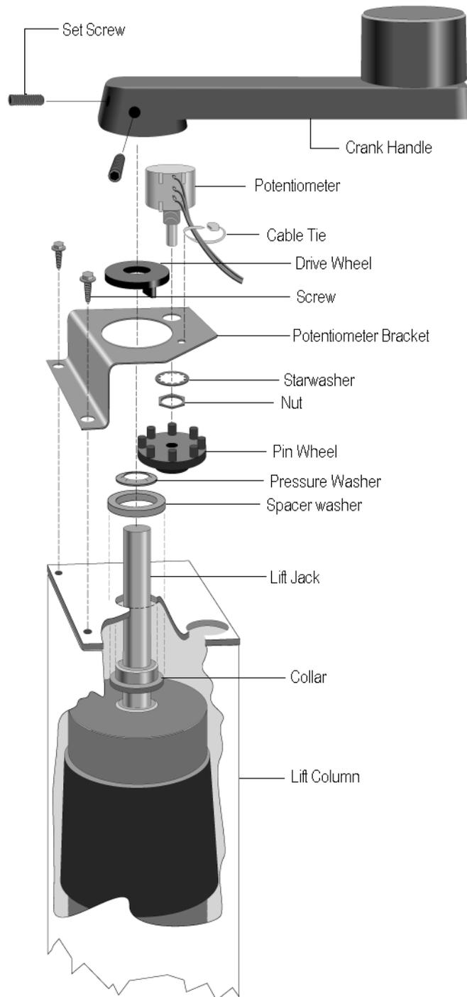
32. Calibrate the lift assembly as described in Procedure 4.1 of this appendix.
